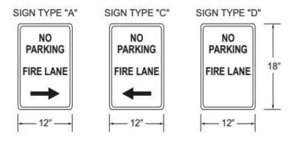
(Reason: Reflects current markings for apparatus access roadways as indicated in the recommended amendment to Section 503.3)
